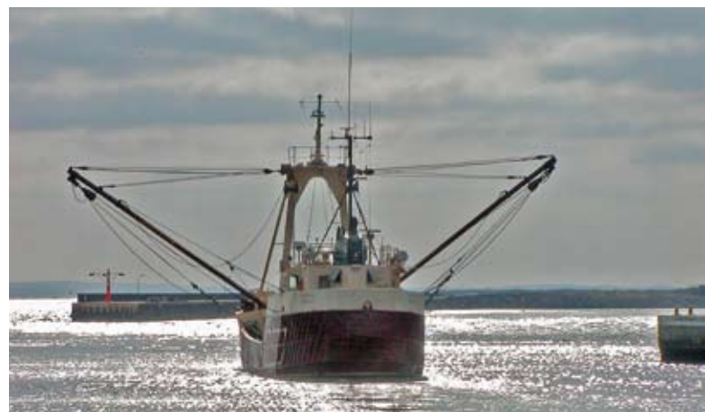
Beam trawler for shrimp fishing leaving the harbour in Havneby, Rømø. Photo: Lars Maltha Rasmussen.
